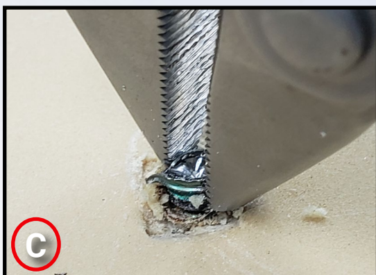
C: Using pliers to try and remove the screw shaft
