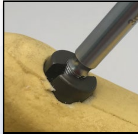
A SHUKLA Screw (S9SCREW) Stripped Screw Extractor attempting to engage with an embedded lag screw.
