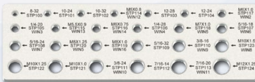
Image 3 Use the Thread Sizing Board to determine the thread size of the IM nail cap. Use the size measurement to select the appropriate threaded extractor tip
