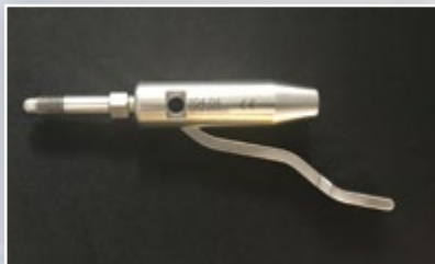
1. Insert cam handle into cam cap, lining up holes.
