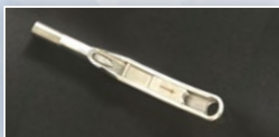
4. Insert curved jaw into curved body. There is an arrow on the jaw to indicate direction.
