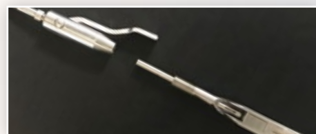
6. Connect the cam cap/handle assembly to the curved body/jaw assembly via the push rod.
