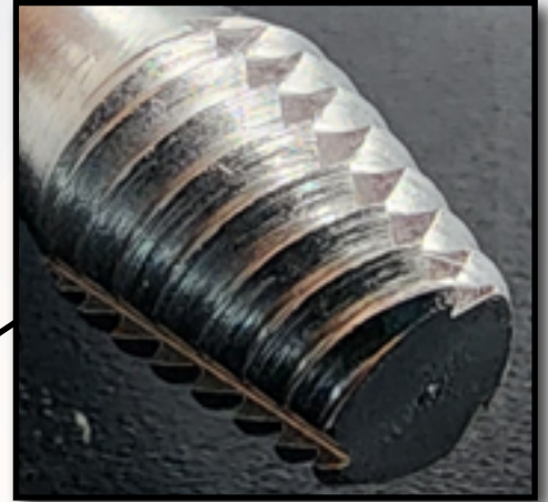
Reverse threading cuts new threads into the wall of the stripped screw well.
