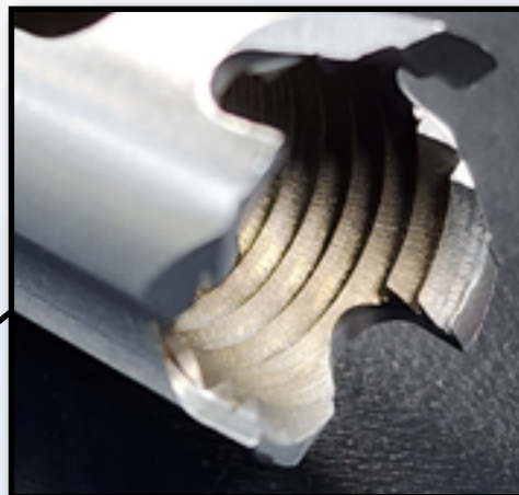
Tapered reverse threads capture the screw quickly while trephine teeth cut through bone.
