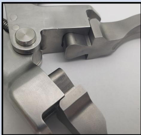
*Dovetail slots in the extractor allow for the rapid insertion of any of the modular glenosphere jaws.*
