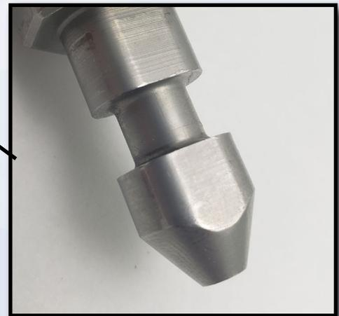
*Quick-connect hub end on the extractor allows for instrumentation to be inserted and removed whenever needed.*
